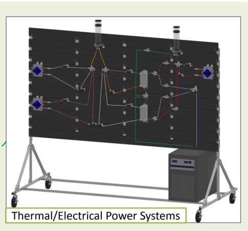
The newest experimental system seeks to emulate the interaction between thermal and electrical systems of an aircraft.
